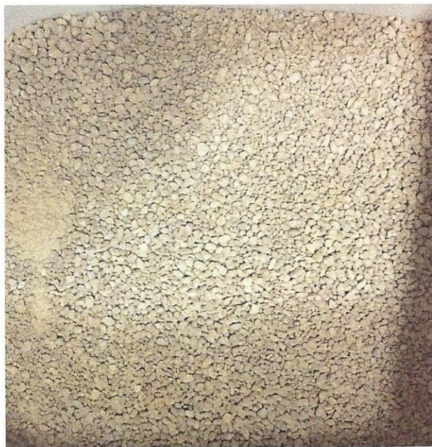
Fig. 5. ProNuCur HY in the container. A mixture of very fine and coarse material. The coarse material would not be appropriate for a golf green.
