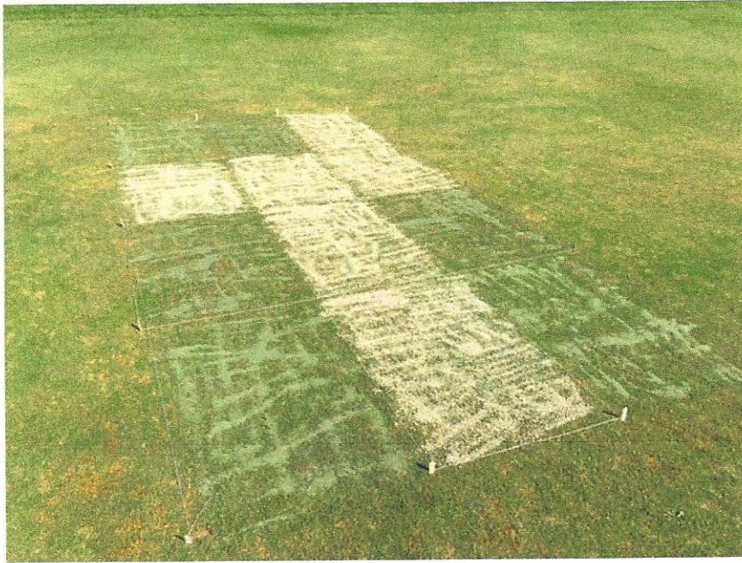
Fig. 6. ProNuCur and sand, after sprinkling on to aerified plots
